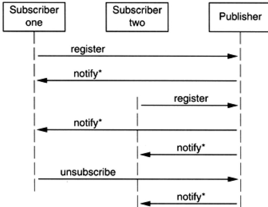
A sequence diagram shows the flow of messages among several objects, with objects arranged in columns. Each message is shown as a labeled arrow from the sender's column to the receiver's column. An asterisk in the label means that more than one message of this type can be sent.
