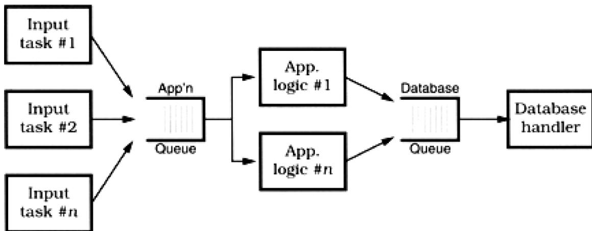
Each box represents a separate process; processes communicate via work queues. Each input process monitors one incoming communication line, and makes requests to the application server. All requests are asynchronous: as soon as the input process makes its current request, it goes back to monitoring the line for more traffic. Similarly, the application server makes requests of the database process,<sup>[5]</sup> and is notified when the individual transaction is complete.
